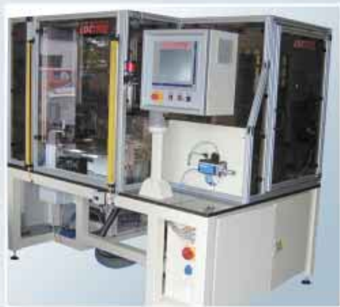
Dispense an UV-curing station for medical bonding application
