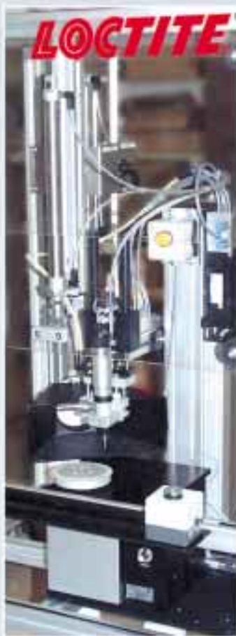
Turntable for bonding of solid gaskets
